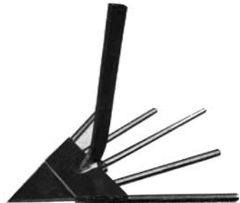
Winged subsoiler used in the Kemink system
